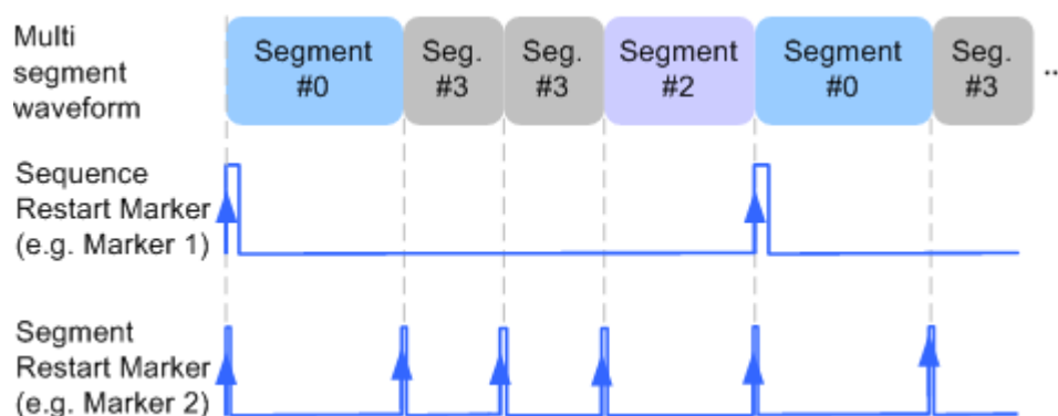
Figure 5-31: Example of marker signals
